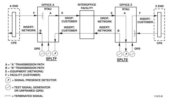
Figure 570-12. Typical Point-to-Point Test Configuration
